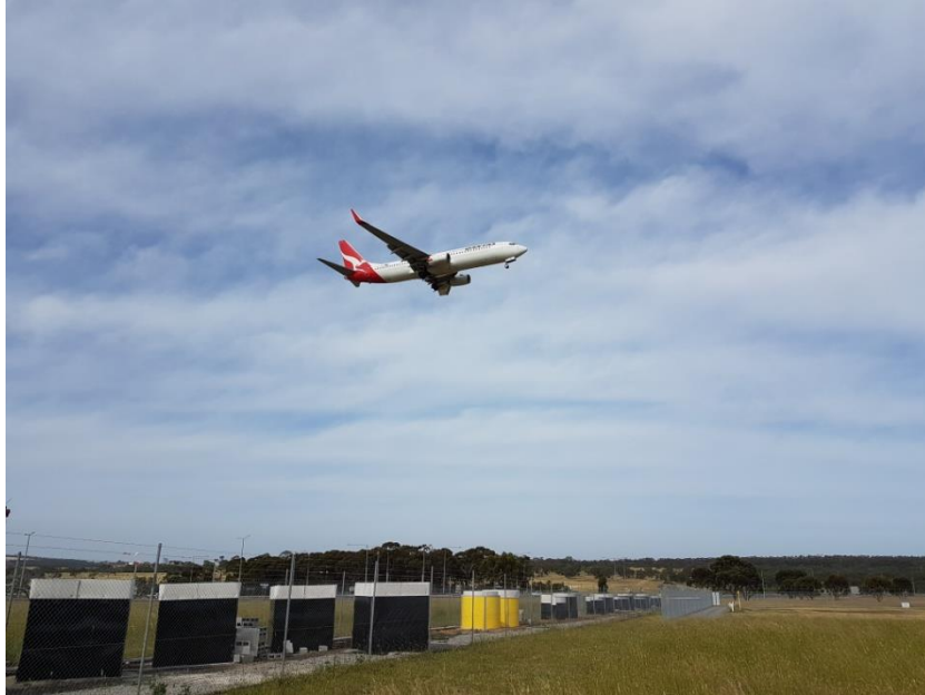
Figure 3. Wake array at Melbourne Airport showing bi-static acoustic transceivers of the 8 used to make wake vortex measurements. The array is set across the 16 approach at 990m from the 16 threshold. The positions of each of the transceivers relative to the centre line is shown in the titles to the 8 transceiver measurements in Figures 5, 11 and 14.
